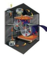
Through-Air Drum Drier Features Diagonally Offset Drums to increase Drying Area.
